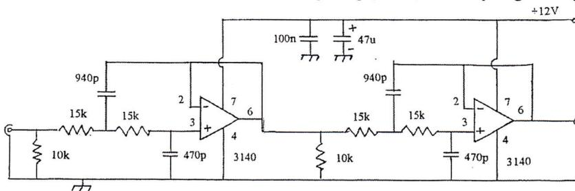
Figure 4. 4<sup>th</sup> order LPF used to tailor the NBTV video baseband
