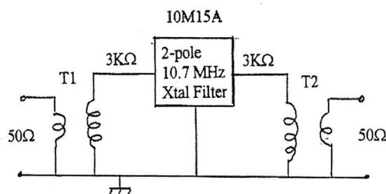
Figure 5. Circuit used for testing crystal filter in a 50Ω system.
