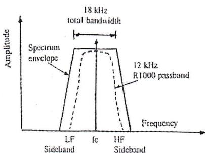
Figure 1. Notional representation of NBTV DSB AM signal spectrum
