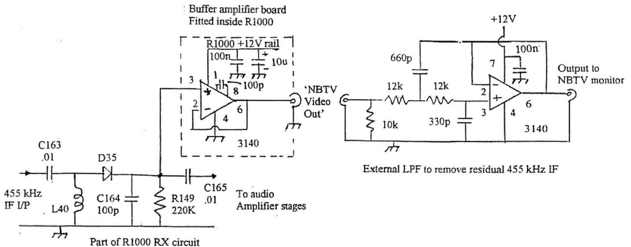
Figure 3. The DC coupled signal take-off from the AM detector diode
