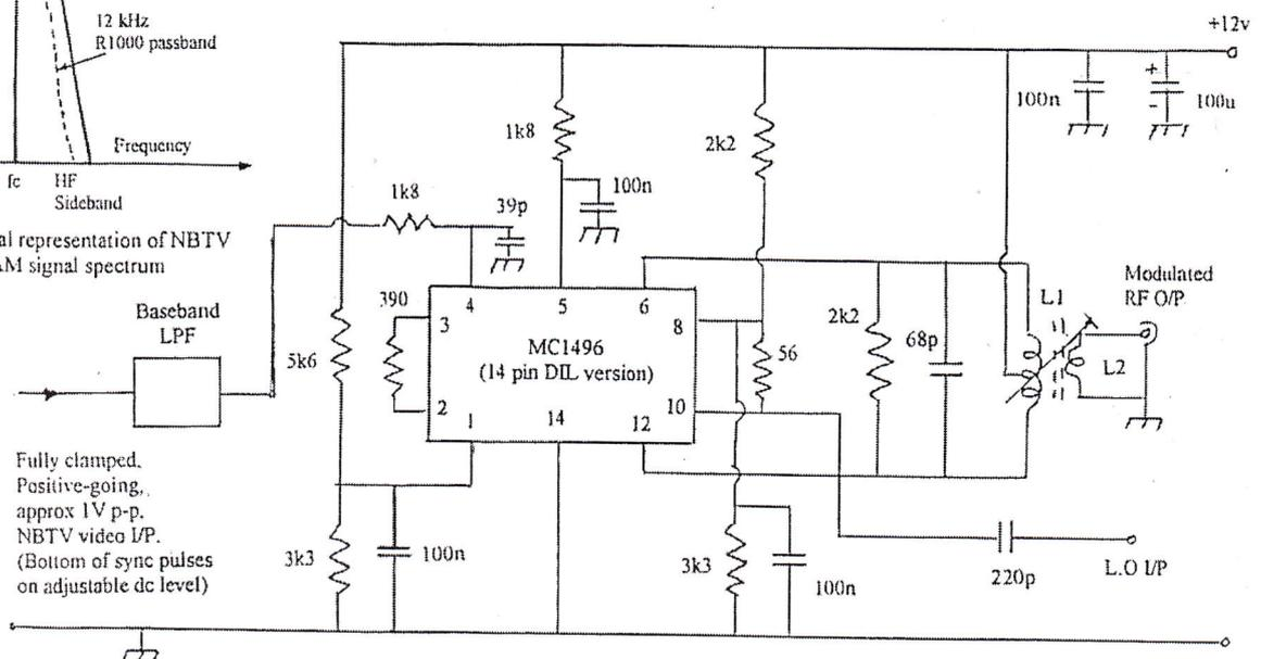
Figure 2. AM modulator circuit used for the experiments.
