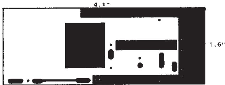
Fig.2 PRINTED CIRCUIT PATTERN (component side)
